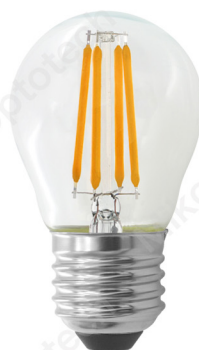
G45 Globe Glass/Warm White LED Filament Voltage: AC 110-240V, 100LM/W Wattage: 3-3.5W Base: E27/ E26 Size: \Phi 45x75mm
